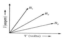
A student carries out an experiment and plots the V-I graph for the three samples of nichrome wire with resistances  $R_1$ ,  $R_2$  and  $R_3$  as shown in the figure. Which of the following is true.
